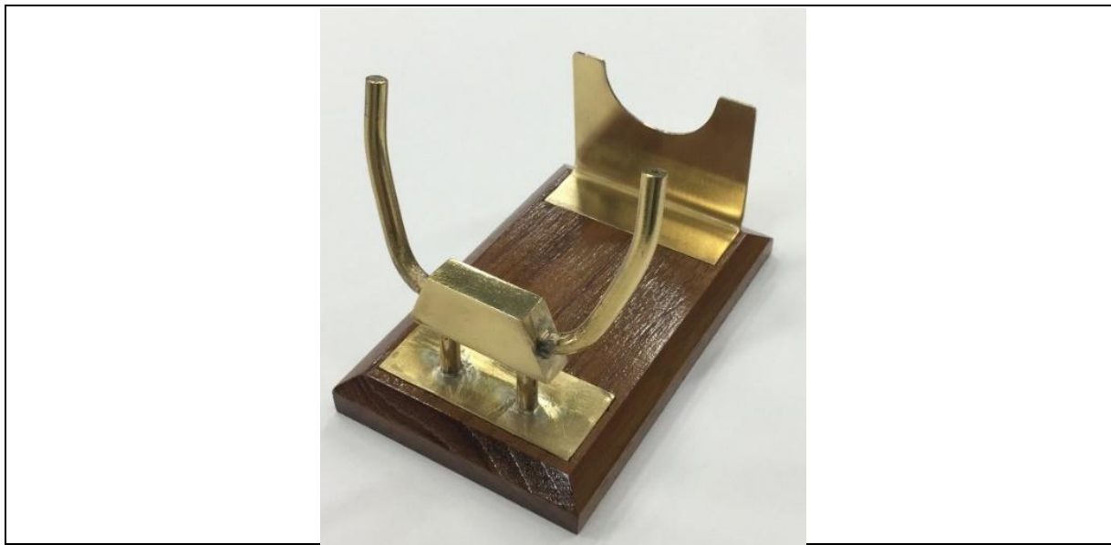
Figure 7: Sample of a final product using brass, with the metal holders attached to a wooden base plate.
