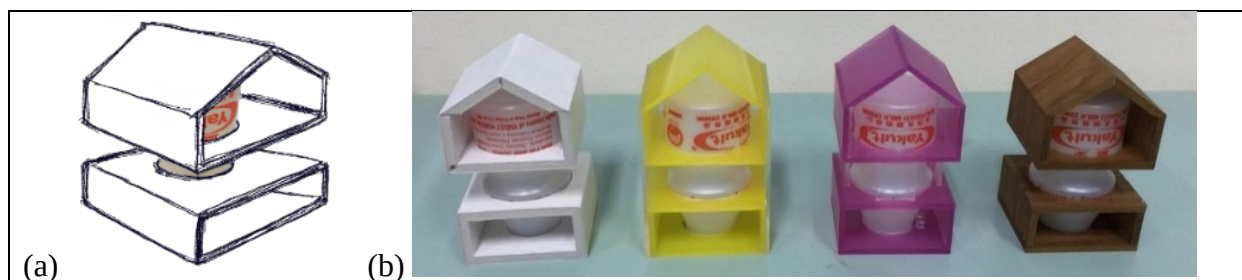
Figure 19: (a) Sixth design. (b) Mock-up and samples using acrylic and teak.
